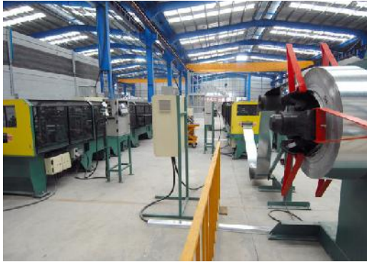
Precision Roll Forming Equipment for Seismic Braced Frame Structural Systems & Roof/Wall Cladding.
